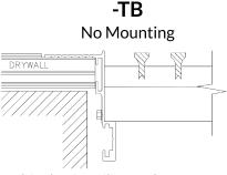
Designed for lay-in ceiling and custom applications. For lay-in, order 2" under to account for flange.
