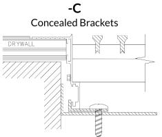
Product is fastened to duct-mounted brackets, which are concealed behind the blades.
