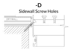
Screw holes are drilled at a 45° angle on inner flange. Only available with Removable Core.
