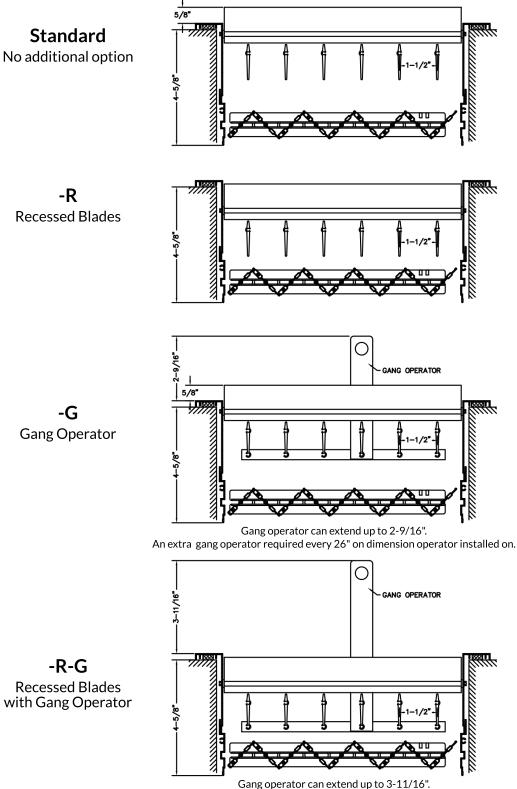
An extra gang operator required every 26" on dimension operator installed on.
