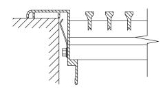
Hidden clips behind the flange to keep the grille secure in the opening. Only suitable for floor & sill applications.
