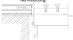
Designed for lay-in ceiling and custom applications. For lay-in, order 2" under to account for flange.
