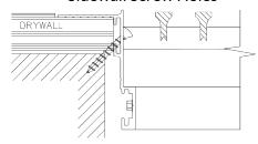
Screw holes are drilled at a 45° angle on inner flange.
