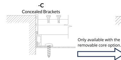
Product is fastened to duct-mounted brackets, which are concealed behind the blades.
