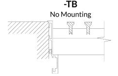
Designed for lay-in ceiling and custom applications. For lay-in, order 2" under to account for flange.
