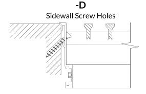
Screw holes are drilled at a 45° angle on inner flange.
