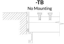
Designed for lay-in ceiling and custom applications. For lay-in, order 2" under to account for flange.
