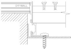
Product is fastened to duct-mounted brackets, which are concealed behind the blades.
