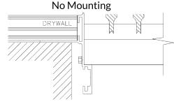
Designed for lay-in ceiling and custom applications. For lay-in, order 2" under to account for flange.
