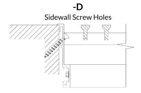
Screw holes are drilled at a 45° angle on inner flange. Only available with Removable Core.
