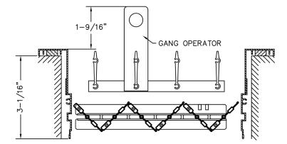
Gang operator can extend up to 1-9/16". An extra operator required to be installed every 26" in length. Only available with -R Recessed Blade option specified.
